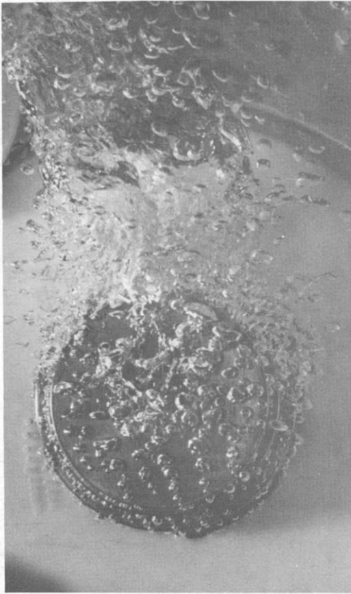
FIG. 10. Front view of 3-disc copper fin in boiling Freon-113. Q = 98 \text{ W} and \Delta T_R = 66.5^\circ\text{C} .
